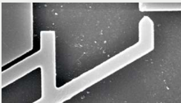
Prototype of a NEM logic switch with zero leakage in the off state due to air gap
